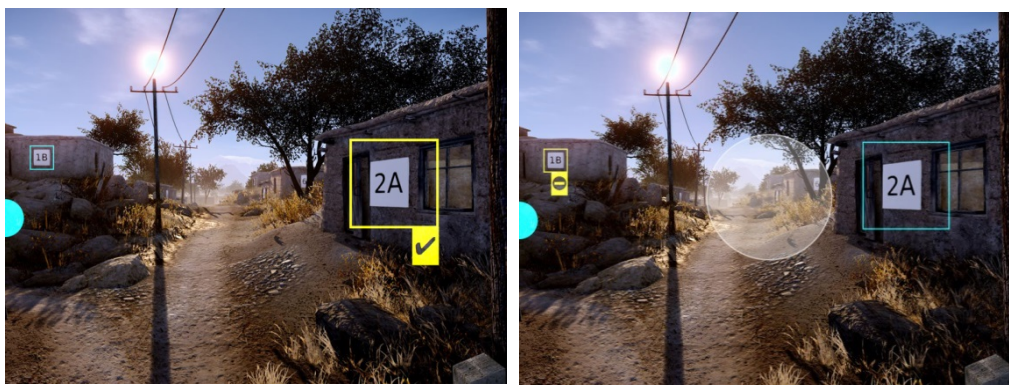
Figure 1: Alphanumeric codes on landmarks are highlighted using a turquoise rectangle in the AR view. A selected rectangle is highlighted in yellow and the symbols for "to edit" (left) and "irrelevant" (right) is displayed on the lower right corner of this rectangle.
