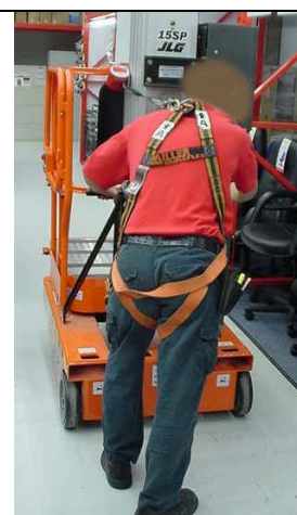
Figure 6: Twisted subpelvic strap. CSST private communication
