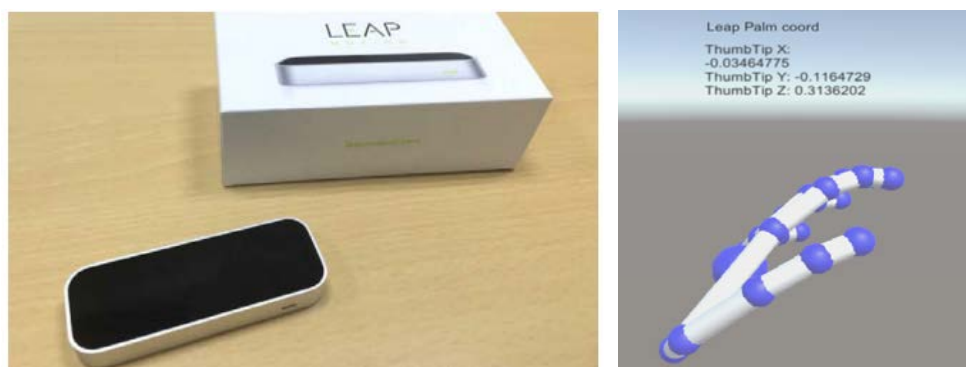
Figure 3: (left) Leap Motion sensor module. (right) While moving one's hand, the (X, Y, Z) coordinates of the thumb tip of the left hand has been recorded at a sampling rate of about 30 Hz.
