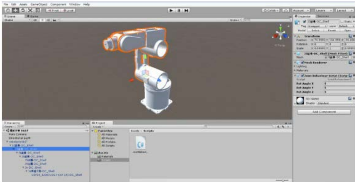
Figure 1: The 6 DOFs robotic arm applied in this trajectory training system (J3 structure)
